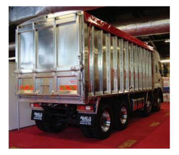
specifying tipper trucks. And hence Aliweld's 7ft 3in Highsider, with 40m<sup>3</sup> capacity and hand welded construction – claimed to be the lightest bulk volume truck body on the market.
